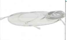
These cables are made of heavy duty 3/16" 7x9 multistrand aircraft style steel cable and are coated with vinyl to prevent scratching of equipment. Every cable has a fitting at each end that allows it to be looped or attached to a lock. Cables can be linked together to create longer lengths.
