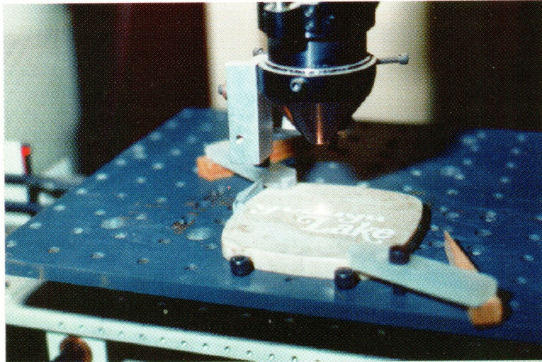
Laser etching example using an MD-2b and an XY-18 positioning table
