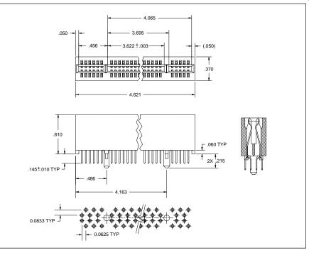
**Figure 1.** The STD 32 connector contacts are arranged as 68 directly opposed pairs. The center section of 57 contact pairs provide backward compatibility with older STD-style cards and expansion to 16-bit non-multiplexed transfers. The remaining 11 contact pairs on the card extensions allow 32-bit non-multiplexed data transfers while maintaining compatibility with older 8-bit STD I/O cards.
