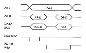
Figure 2. 16-Bit Data Multiplexing.
