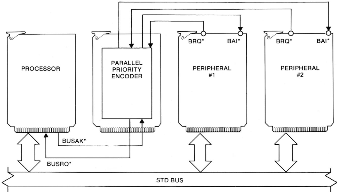
Figure 2-7. Parallel Scheme for Bus Priority
