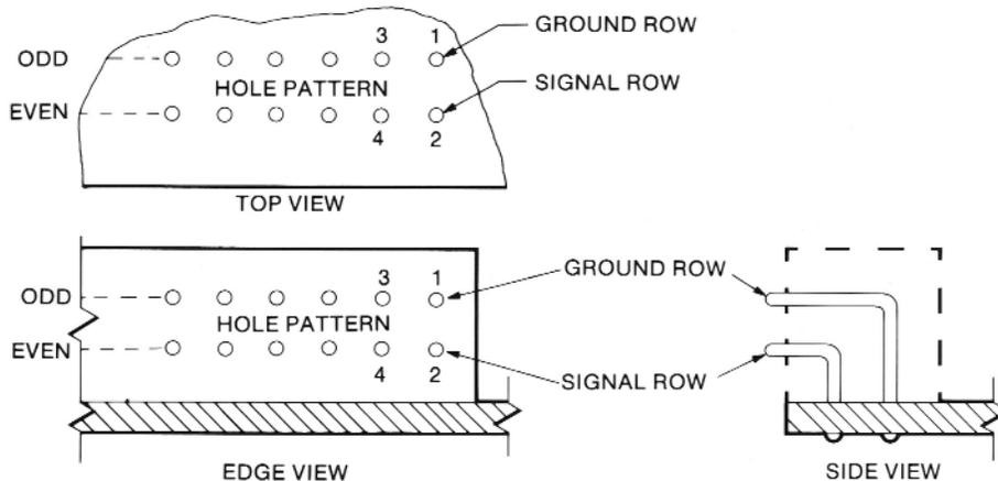
Figure 2-3. Recommended Connector Arrangement for Priority Encoder Cards
