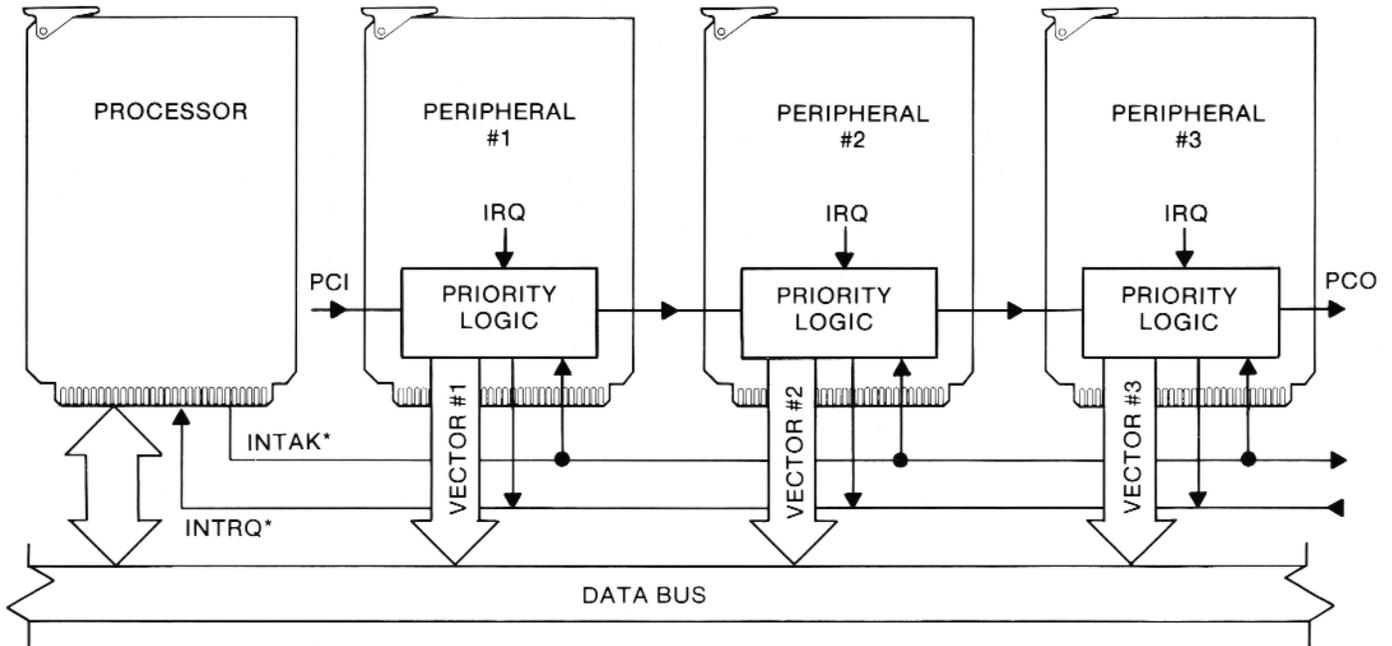
Figure 2-1. Serial Scheme for Interrupt Priority
