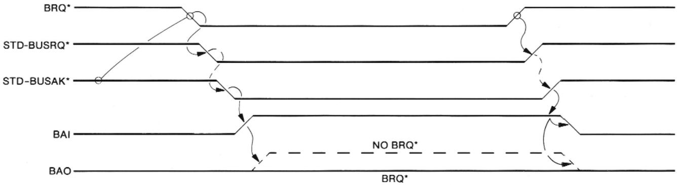
Figure 2-5. Serial Priority Signal Sequence
