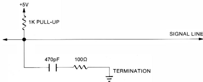
Figure 2-13. Passive AC Termination and Signal Pull-Up
