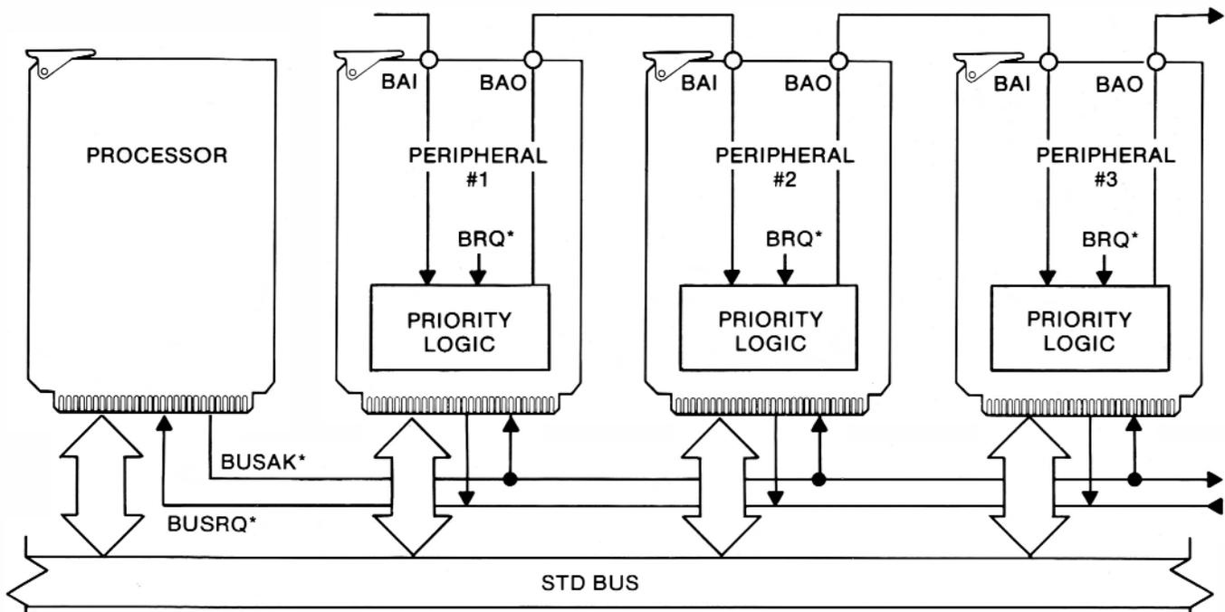
Figure 2-4. Serial Scheme for Bus Priority
