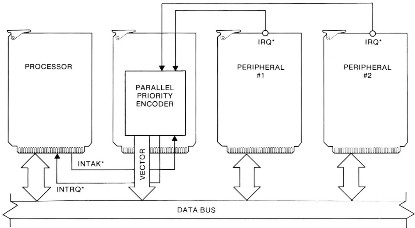
Figure 2-2. Parallel Scheme for Interrupt Priority
